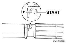
(4) Pull the manual starter handle slowly until you feel resistance. Then give a strong pull straight out to crank and start the engine.
