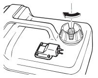
(3) Disconnect the fuel line if you are using an external fuel tank.
