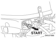
(5) Pull the manual starter handle slowly until you feel resistance. Then give a strong pull straight out to crank and start the engine.
