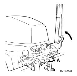
(3) Hold the handgrip and steering bracket as shown in the illustration and lift up the outboard motor using two people.
