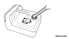
(9) Tighten the filler cap securely.
