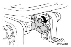
(3) Slightly tilt the outboard motor up. The tilt support bar will lock automatically, supporting the outboard motor in a partially raised position. This outboard motor has 2 positions for shallow water cruising.
