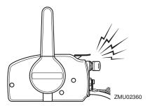
If the alert system has activated, stop the engine as soon as it is safe to do so. Check the oil level and add oil as needed. If the oil level is correct, consult your Yamaha dealer.
