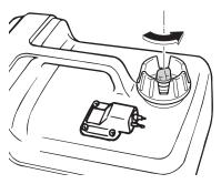
(2) If there is a fuel joint on the motor, align the fuel joint on the fuel line with the fuel joint on the motor and firmly connect the fuel line to the joint while pinching the joint. Then firmly connect the other end of the fuel line to the joint on the fuel tank.
