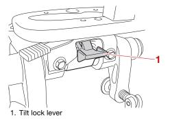
To lock it, set the tilt lock lever in the lock position. To release, push the tilt lock lever in the release position.
