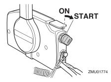
(7) Immediately after the engine starts, release the main switch and allow it to return to "ON" (on). The remote choke system stops operating when the main switch is released. NOTICE: Never turn the main switch to "START" (start) while the engine is running. Do not keep the starter motor turning for more than 5 seconds. If the starter motor is turned continuously for more than 5 seconds, the battery will be quickly discharged, thus making it impossible to start the
