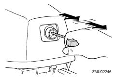
(6) After the engine starts, slowly return the manual starter handle to its original position before releasing it.
