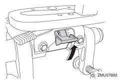
(2) Slightly tilt the engine up until the tilt support bar is automatically released. (3) Slowly tilt the engine down.
