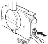
(2) After stopping the engine, tighten the air vent screw on the fuel tank cap and set the fuel cock lever or knob to the closed position, if equipped.
