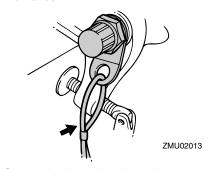
(3) Secure the clamp bracket to the transom using the bolts provided with the outboard (if packed). For details, consult your Yamaha dealer. WARNING! Avoid using bolts, nuts or washers other than those contained in the engine packaging. If used, they must be of at least the same quality of material and strength and must be tightened securely. After tightening, test run the engine and check their tightness.
