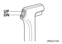
To raise the bow ("trim-out"), tilt the outboard motor up.
