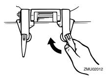
(2) If the restraint cable attachment is equipped on your engine, a restraint cable or chain should be used. Attach one end to the restraint cable attachment and the other to a secure mounting point on the boat. Otherwise the engine could be completely lost if it accidentally falls off the transom.
