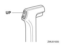
(3) To return the outboard motor to the normal running position, press the power tilt switch and slowly tilt the outboard motor down. EMU28196
