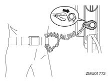
(3) Turn the main switch to "on" (on).
