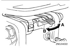
If the resistance does not increase even when the lever is turned to the port side "A", make sure that the nut is tightened to the specified torque.
