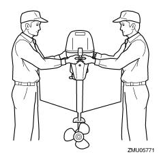
(4) Mount the outboard motor on the center line (keel line) of the boat, and ensure that the boat itself is well balanced. Otherwise the boat will be hard to steer. For boats without a keel or which are asymmetrical, consult your dealer.
