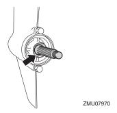
Check the propeller shaft oil seal for damage.
