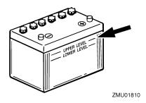
(2) Check the battery's charge. If your boat is equipped with the digital speedometer, the voltmeter and low battery alert functions will help you monitor the battery's charge. If the battery needs charging, consult your Yamaha dealer. (3) Check the battery connections. They should be clean, secure, and covered by an insulating cover. WARNING! Bad connections can produce shorting or arcing and cause an explosion. [EVMID1913]
