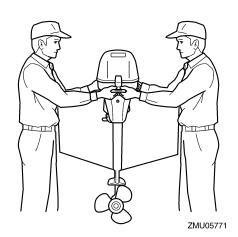
(7) When transporting or storing the outboard motor while removed from a boat, keep the outboard motor in the attitude shown or use an outboard motor stand.
